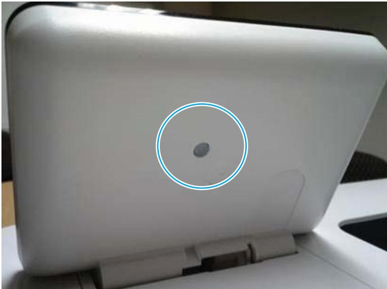
2. Press the diagnostics-access button. Repeatedly pressing the button cycles through the available diagnostics.
