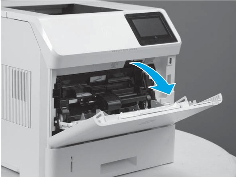
2. Rotate the spring-loaded cover downward to gain access to the separation roller.
